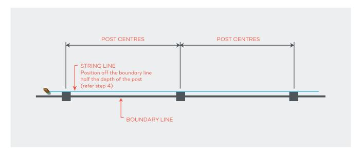
Determine your post hole centres using the table on the next page as a guide and mark out your post hole positions on the ground with line marking paint.
