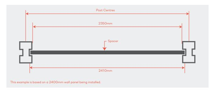
Now insert the next post in the hole using the 'spreader bar' as a spacer. This spacer bar should rest on the base brackets.
